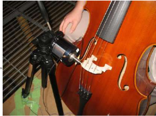
Fig. 7 Configuration of driving the bridge with a mini-shaker.
