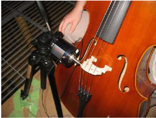
Fig. 4 Configuration of driving the bridge with a mini-shaker.
